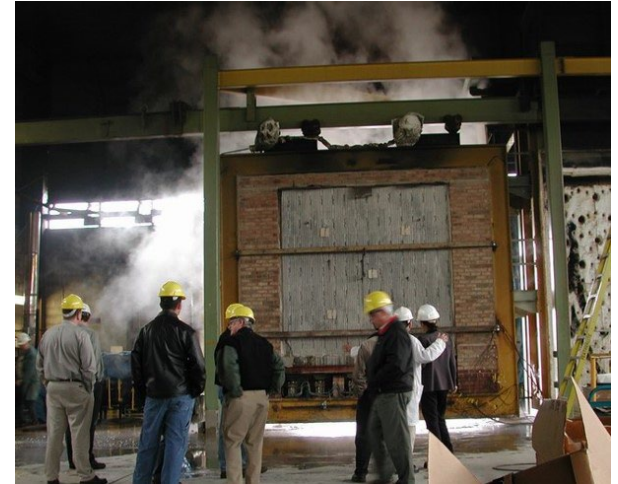
UL - ASTM E119 Testing of ICF Assembly
